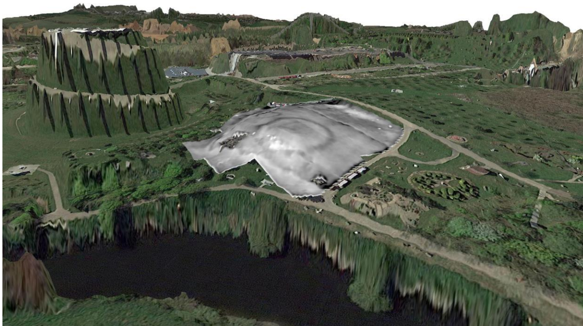
Figure 20. The resistivity survey draped over the Lidar image, height exaggerated 10x to demonstrate the artificially raised platform.
